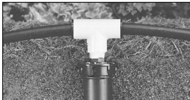
Rain Bird 1800-RETRO provides 200-mesh filtration and 30-psi pressure regulation as a point-of-connection for LD tubing.
